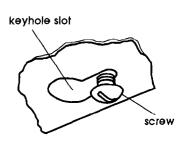
Start screws through neck of each of the four keyhole mounting screw slots marked on the cabinet bottom.
